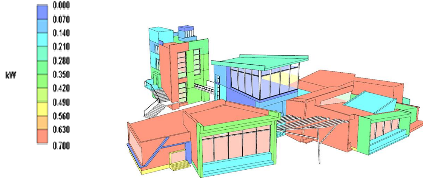
Heating plant sensible load
